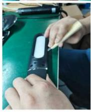
7. 用螺丝刀<u>取下灯板螺丝</u> Use a screwdriver to remove the screw of the LED module
