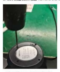
3.拆掉底座里电路板固定支架 Remove the fixing bracket of PCB in the base
