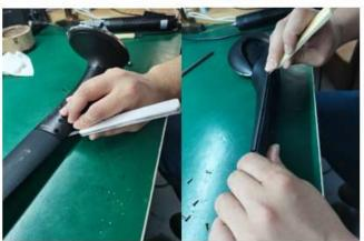
5. 用螺丝刀取下屏幕显示控制电路板 Use a screwdriver to remove the control PCB of the screen display
